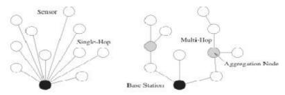
Figure 1.4 Single-hop versus multi-hop communication in sensor networks
